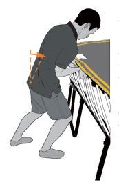
3 Push forward rocking from your heels to the balls of your feet, using the weight of your body to push the white mat rod into the mat rod holder while you keep the mat edge horizontal with your other hand
