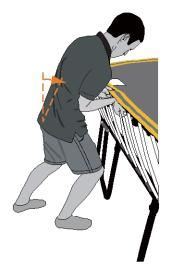
3 Push forward rocking from your heels to the balls of your feet, using the weight of your body to push the white mat rod into the mat rod holder while you keep the mat edge horizontal with your other hand
